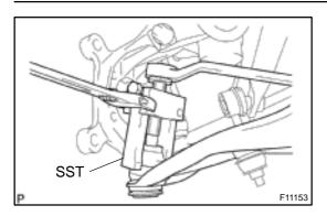
(b) Using SST, disconnect the lower suspension arm from the steering knuckle.
